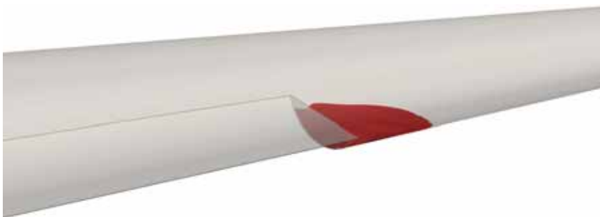
Figure 1: Sudden expansion geometry used in case study simulations, with red clot grown in recirculation region at Re = 388 . Flow is from left to right.
