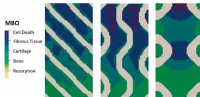
Figure caption: Section cut of 70% porosity scaffold-substrate FE models, considering the MBO for 20s compression time and 6% compression magnitude. Left to right: SD70-SG70-SP70.
