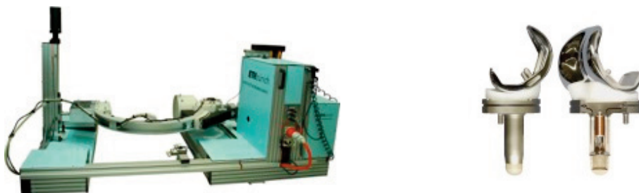
Figure 1: The moving fluoroscope (left) allows the capture of skeletal kinematics throughout complete cycles of daily activities including walking, ramp descent and stair descent. Internal joint contact forces were captured using telemetric prostheses (right), implanted in 6 subjects.
