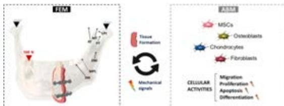
**Figure 1:** Bone healing model: (left) FEM with boundary conditions; (right) ABM with cellular phenotypes and activities.
