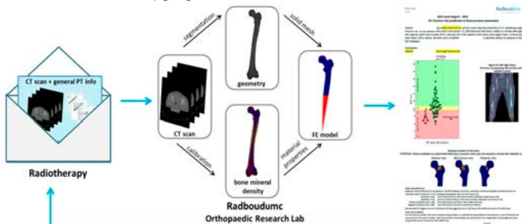
**Figure 1:** BOS workflow. The radiotherapy planning QCT scan is digitally sent, together with some general patient information such as body weight, to our research lab. The CT scan is used to generate the FE model, on which an axial load is simulated until failure. The BOS score is calculated by normalizing bone strength by body weight. Subsequently, a report is returned, which can be used to determine the best treatment for patients..
