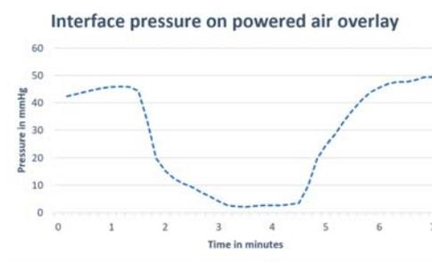
Figure 2. Sacral interface pressure on the low profile, powered air overlay.
